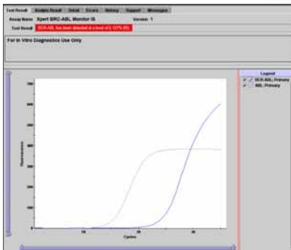
GeneXpert Dx System – Detailed View Results window, both a not detected and positive result. The delta CT value is used in conjunction with a lot specific PCR efficiency value and an assay-specific conversion factor provided to calculate the percent BCR-ABL/ABL to International Scale (%IS).
